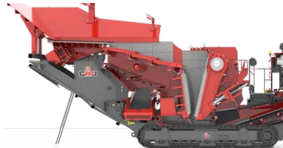
FEED VARIANT WITH LONG PRE-SCREEN
