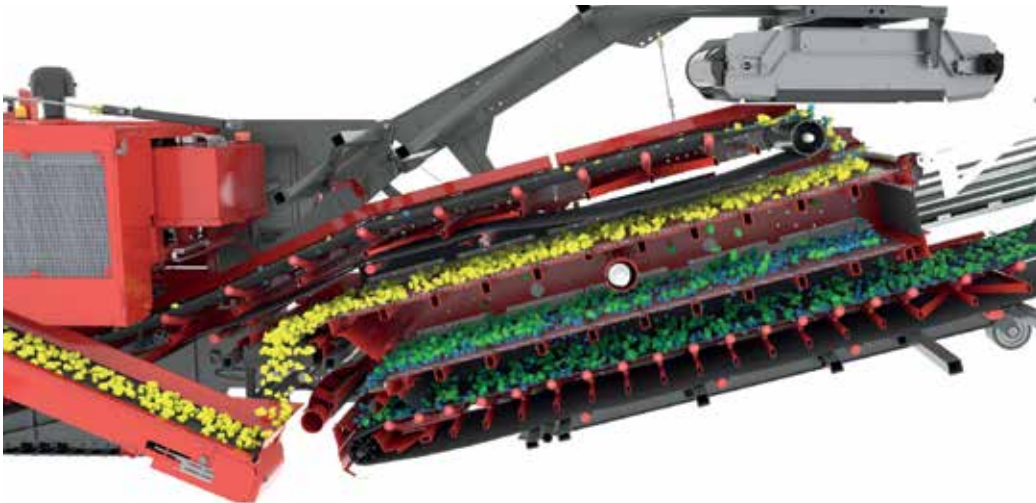
2-DECK WITH SCREEN DECK COMBINATION
