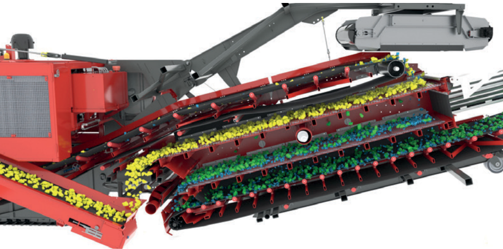
2-DECK WITH SCREEN DECK COMBINATION
