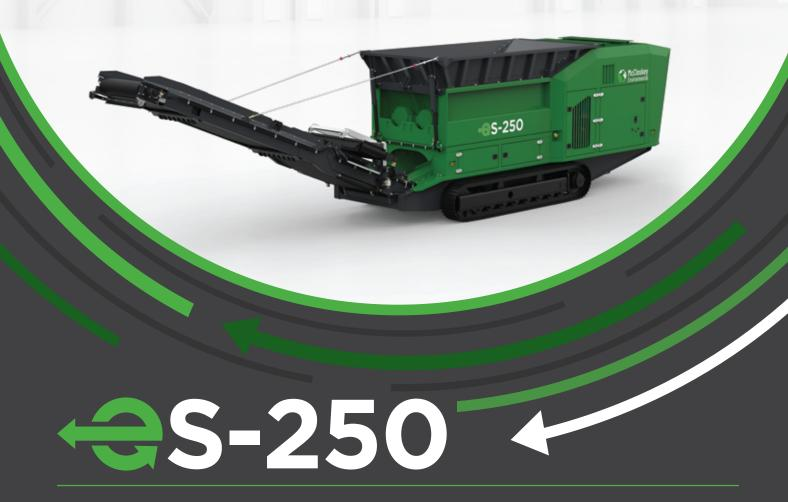
The ES-250 is a tracked primary shredder capable of effectively and reliably shredding virtually any type of material. Designed to meet the needs of plants in which the incoming materials vary greatly in terms of size, composition, and difficulty to shred.
